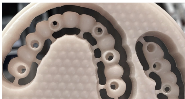
Figure 14: Provisional bridge is milled from a solid PMMA puck (Telio)
